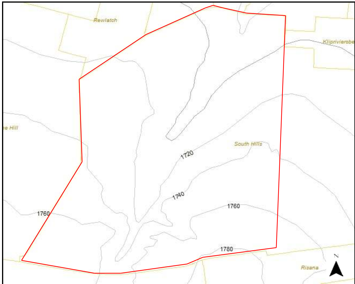
Figure 6: Contour map (20m) indicating the ridges on the southern part of the site and the valley bisecting the site.
