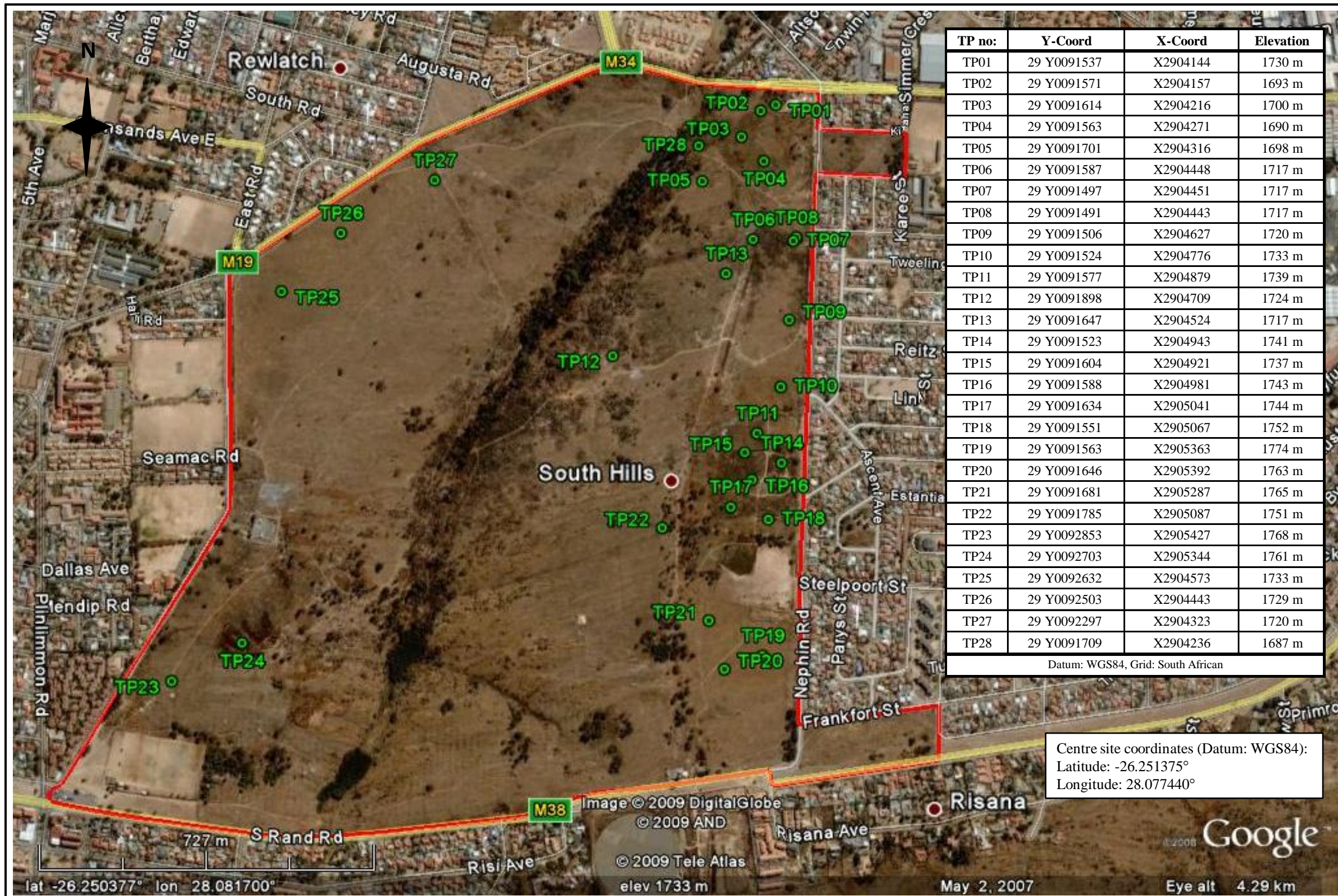
Figure 7: Test pit positions: South Hills - Klipriviersberg Estate
